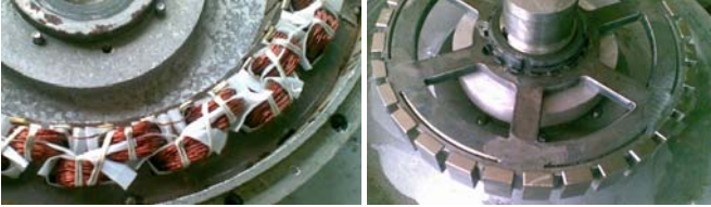
Fig. 9. Stator and rotor details of the manufactured prototype
